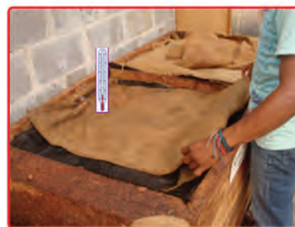
Figure 9. The measurement of fermentation temperature. The temperature of fermentation should be monitored periodically so that in the event of deviations in temperature, a process improvement action can be done immediately.
