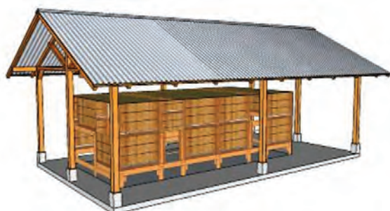
Figure 5. Visualization of Farmer scale fermentation box design.
